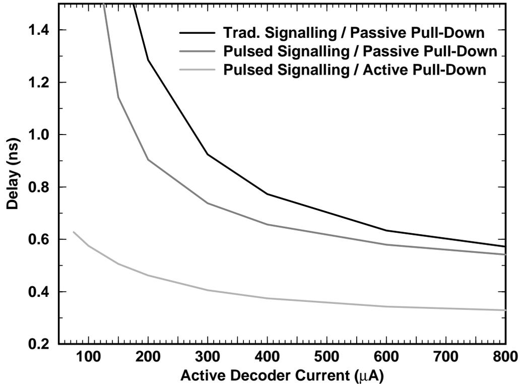
Figure 3-10 Advantages of Pulsed Signalling for Diode Decoders
