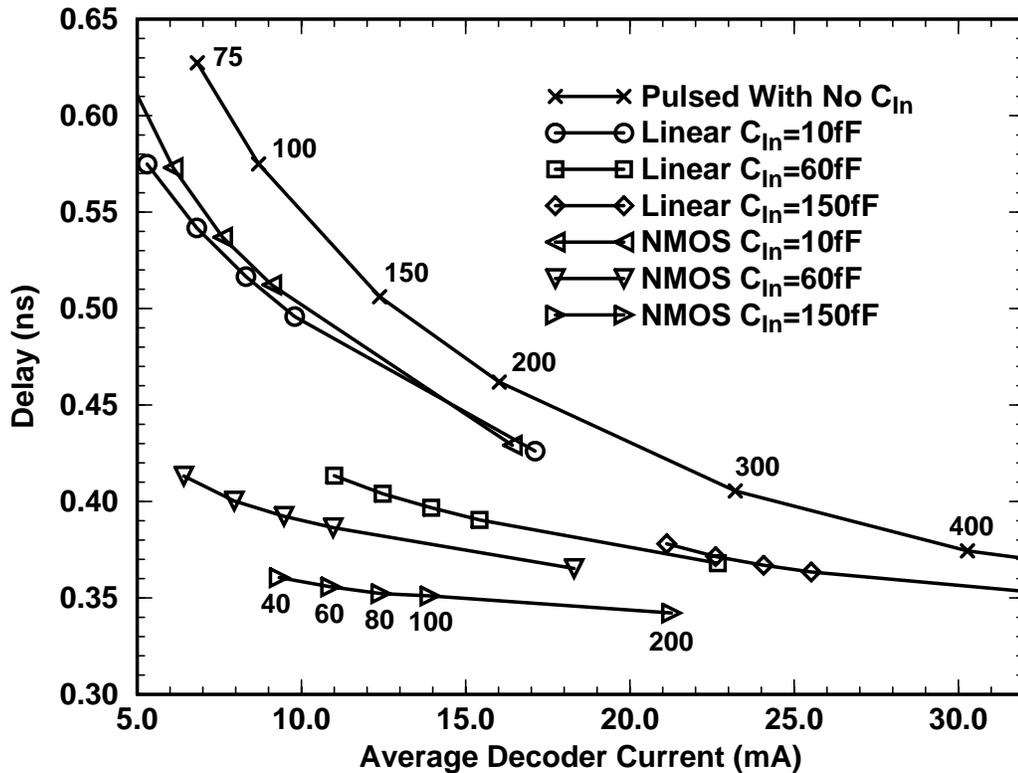
Figure 3-14 Power/Delay Comparison of Pulsed Diode Decoders
