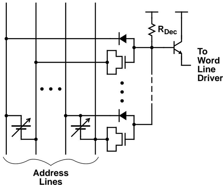
Figure 3-12 A NMOS Capacitor Pulsed Diode Decoder
