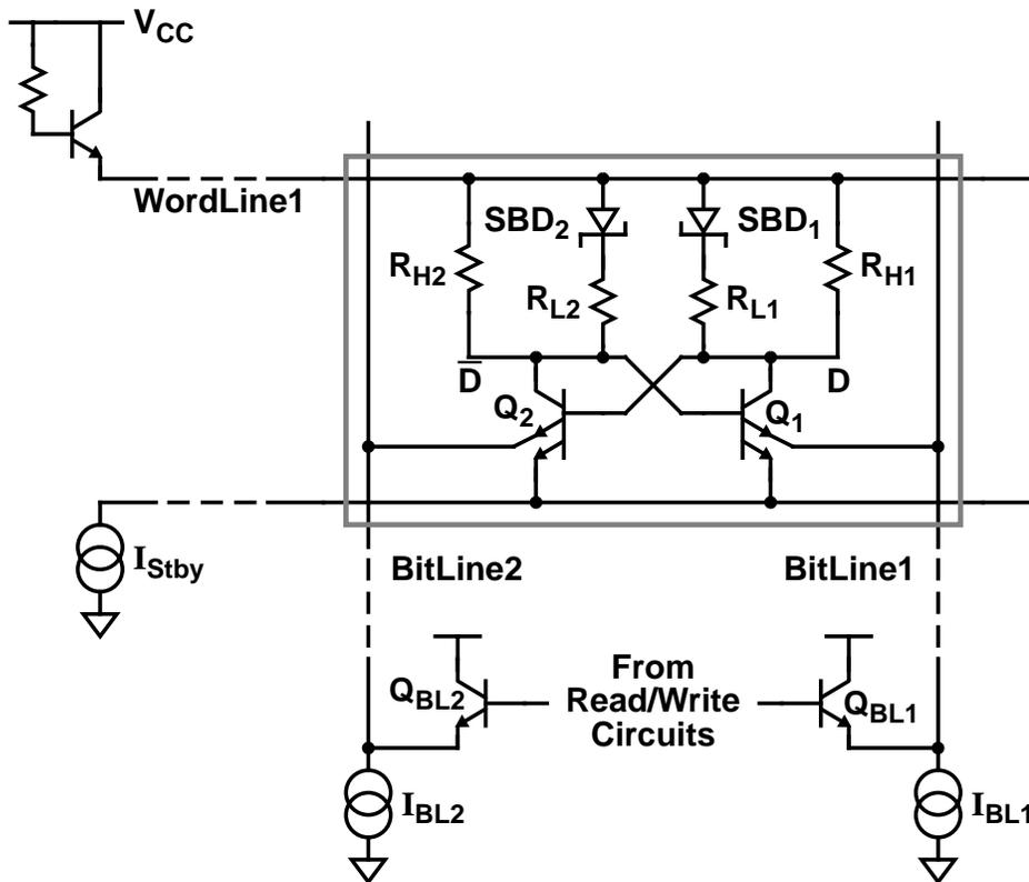
Figure 2-9 Schottky Barrier Diode Load Memory Cell
