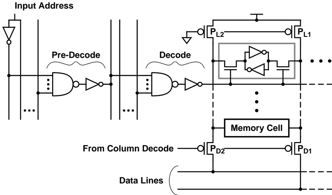
Figure 2-7 Simplified CMOS SRAM Read Access Path
