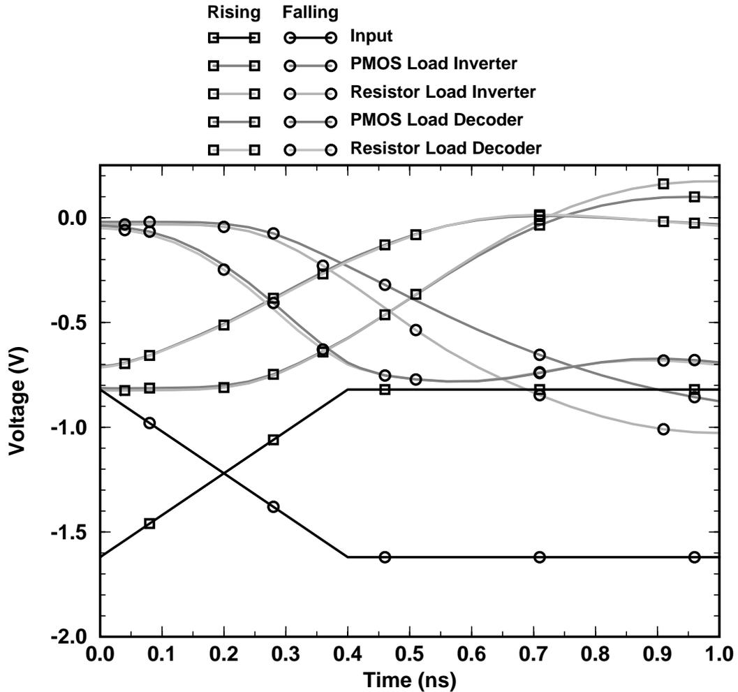
Figure 3-7 Gate Switching Waveforms for PMOS Loads
