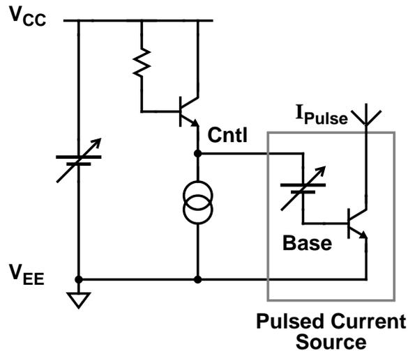
Figure 3-16 Variable Level Shift for Pulsed Current Sources
