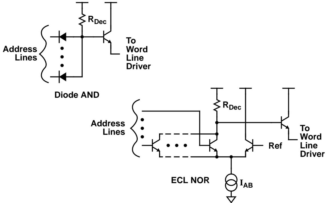
Figure 2-10 Bipolar Decoders
