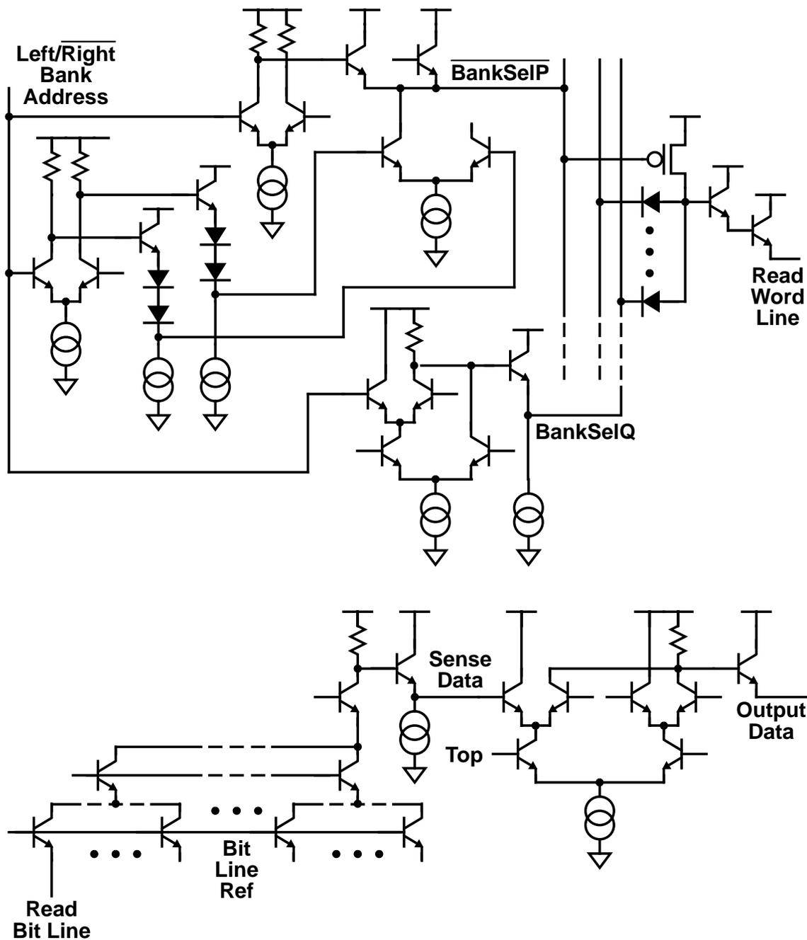
Figure 5-4 Critical Access Path for 16Kx4 SRAM
