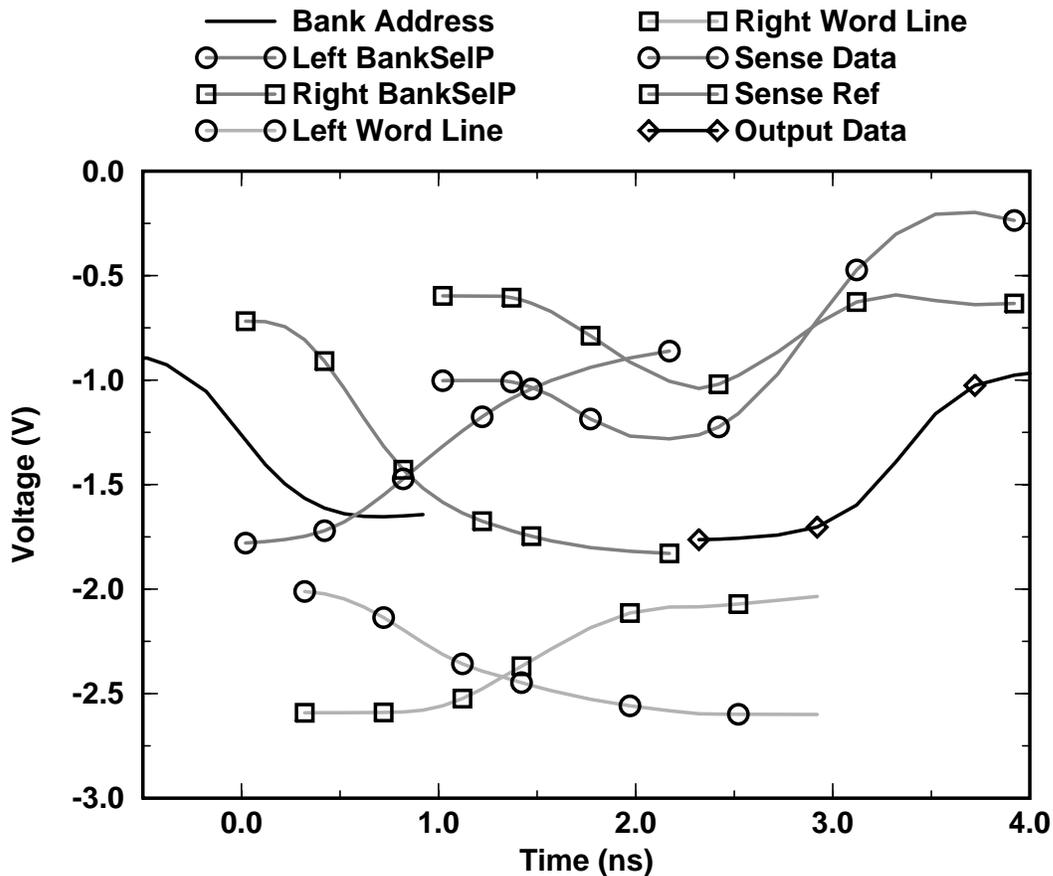
Figure 5-9 Simulated Switching Waveforms for 64K×4 SRAM
