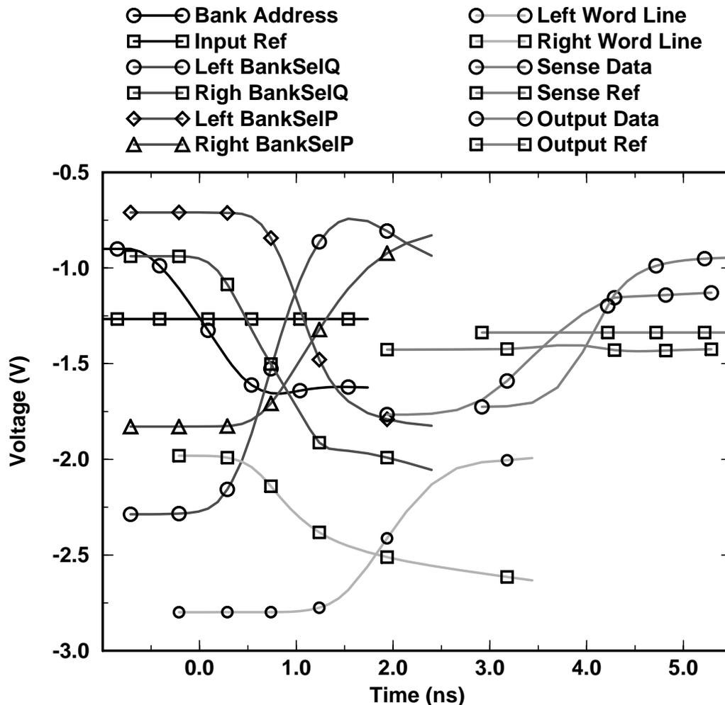
Figure 5-7 Simulated Switching Waveforms for 16K $\times$ 4 SRAM
