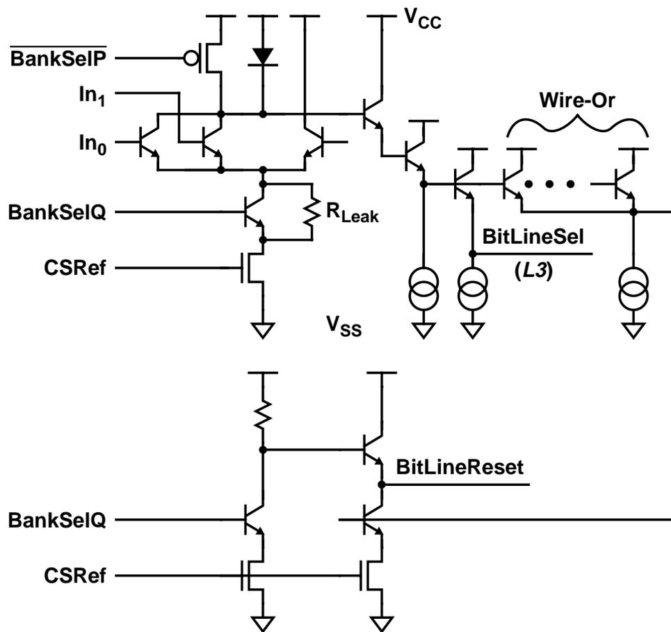
Figure 4-16 Pulsed Bit Line Control Circuits
