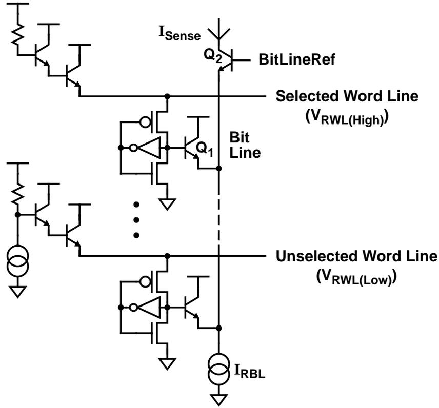
Figure 4-3 CSEA Cell Bit Line Sensing Model
