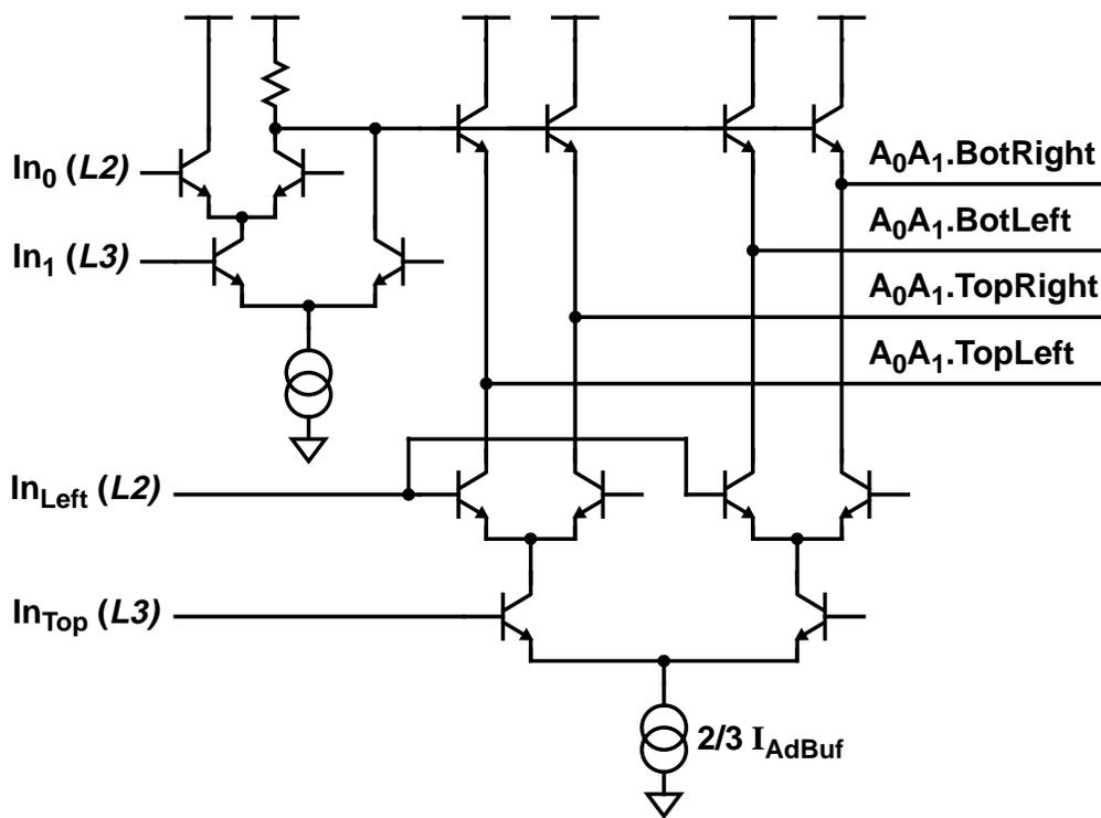
Figure 3-9 Address Buffer with Segmented Address Lines
