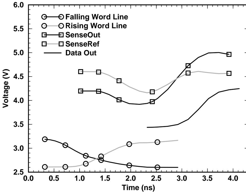
Figure 4-10 Sense Path Performance with Supply Noise
