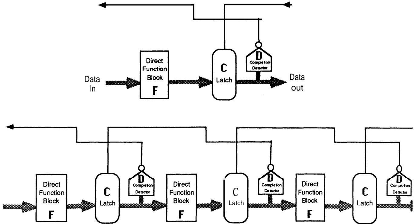
Figure 19: Schematic for stage style **FCO** and a short pipeline composed using that configuration.
