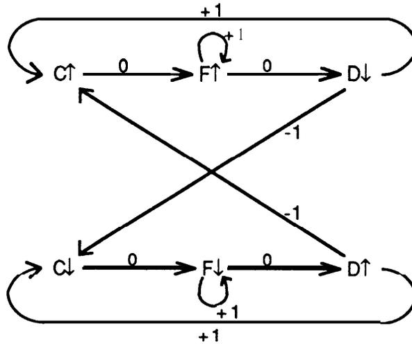
Figure 8: The Dependency Graph for the **PC0** configuration style pipeline can be folded together if the stages are identical to make the Folded Graph shown here.
