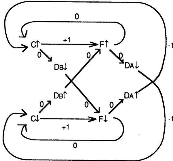
Figure 15: The Folded Dependency Graph for the **PS1** configuration pipeline
