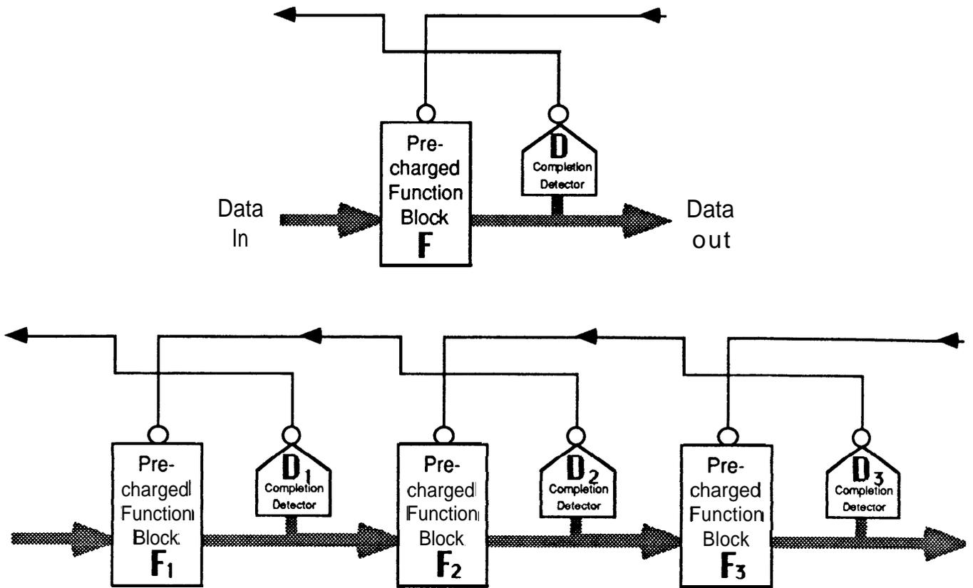
Figure 12: Schematic for stage style **PS0** and a short pipeline composed using that configuration.
