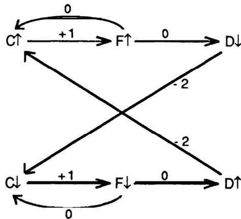
Figure 18: The Folded Dependency Graph for the **CFO** configuration pipeline
