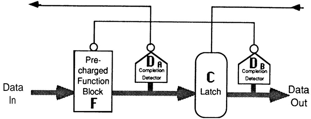
Figure 14: Schematic for stage style **PS1**
