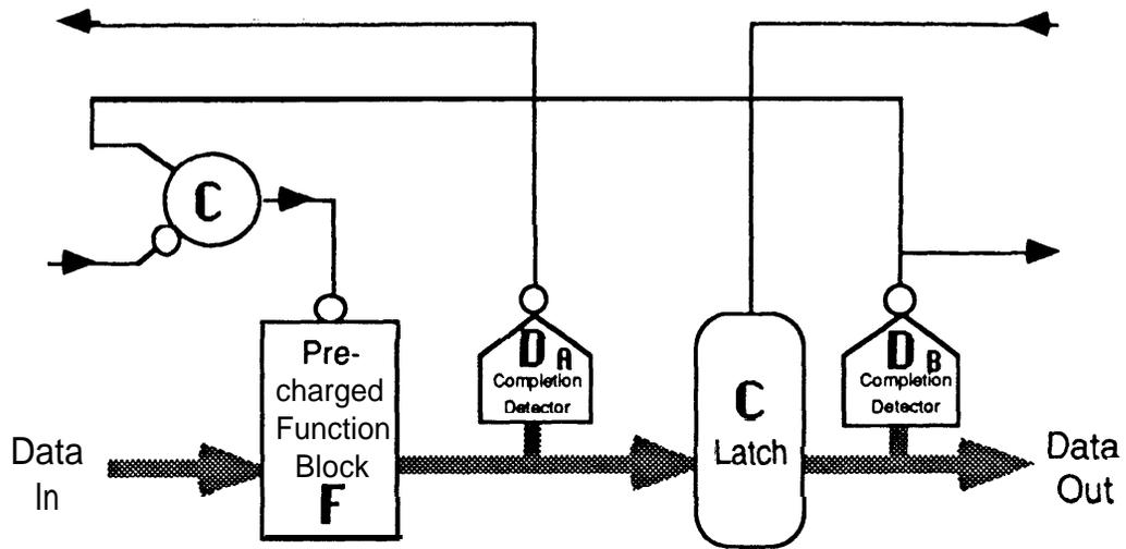
Figure 9: Schematic for stage style **PC1**
