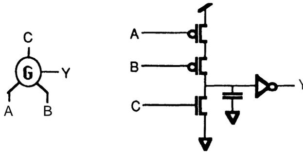
Figure 5: A “Generalized C-element” may have different signals triggering the rise and fall of the output. This figure shows a Generalized C-element with one input on the top to trigger the rising output transition, and two inputs on the bottom required for the falling transition.
