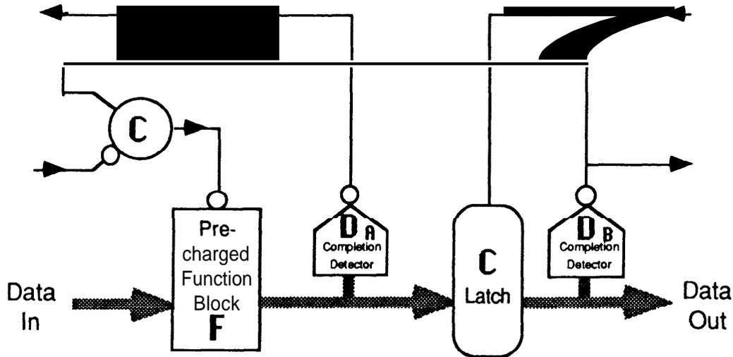
Figure 21: Schematic for stage style **PL1**.
