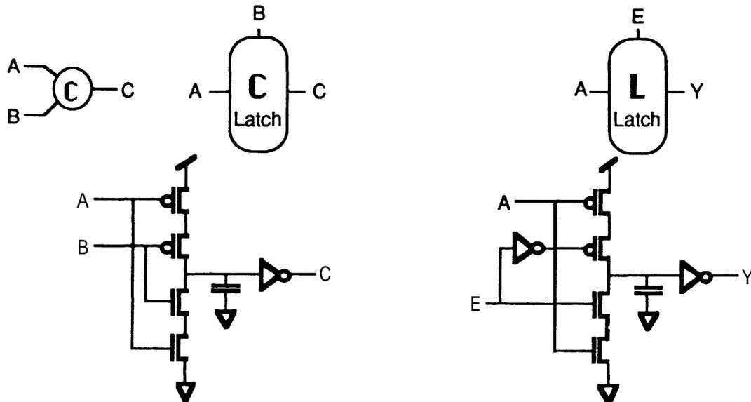
Figure 4: CMOS implementations of a C-element (or C-latch) and a standard flow latch.
