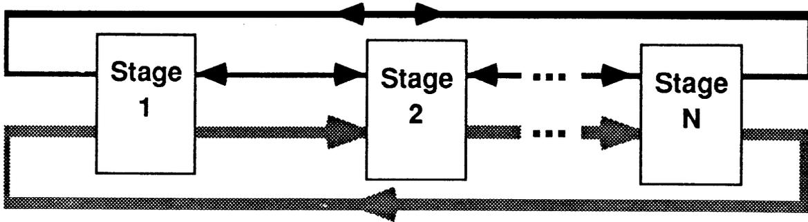
Figure 2: A self-timed ring is a loop of stages containing one or multiple tokens flowing around without intervention from external control except during initialization.
