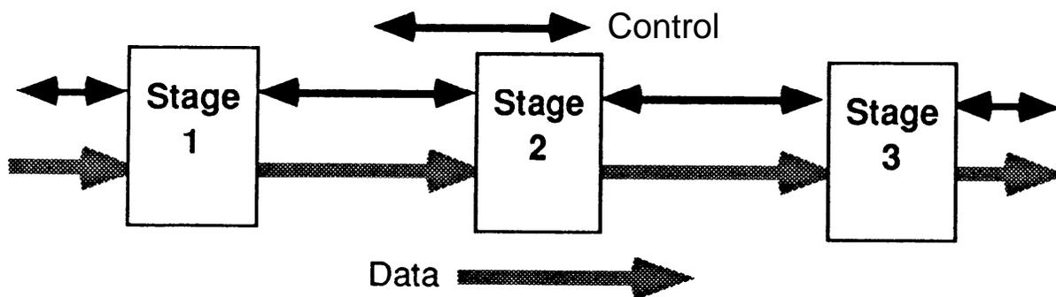
Figure 1: Overall structure of a pipeline is a linear sequence of stages
