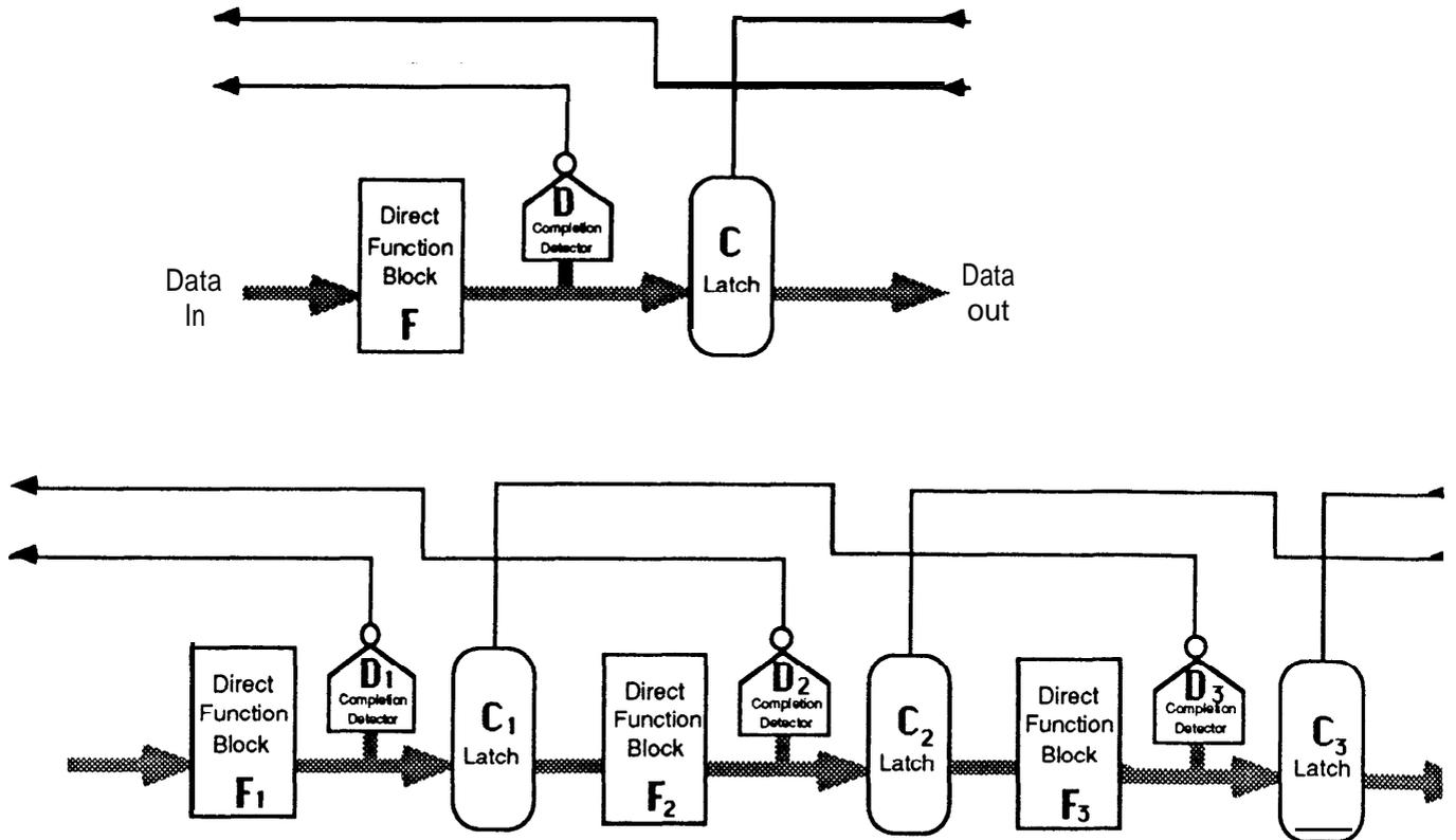
Figure 17: Schematic for stage style **CFO** and a short pipeline composed using that configuration.
