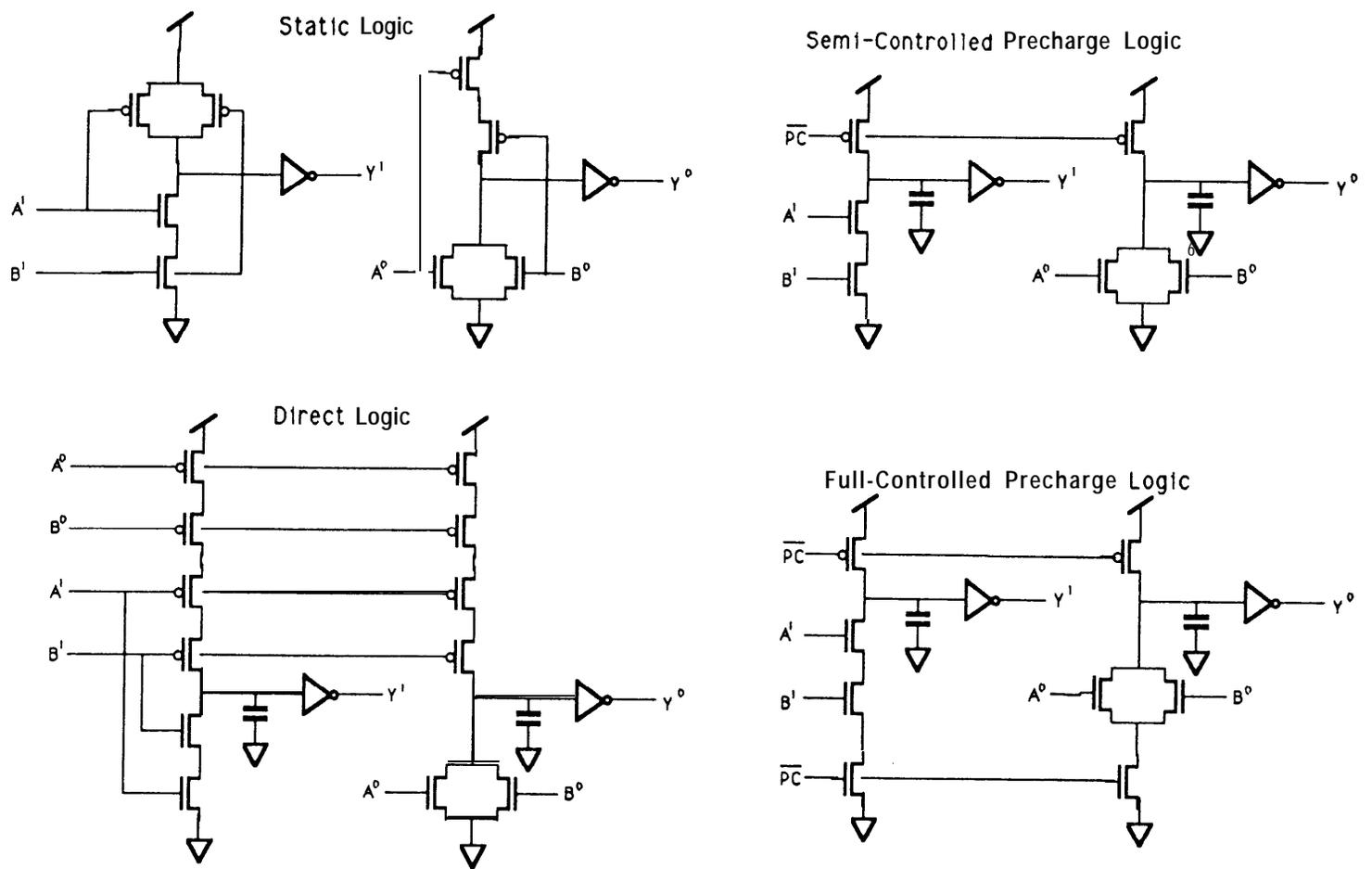
Figure 3: Four possible Function block styles to generate dual-monotonic outputs: Static logic, Direct Logic, Semi-controlled Precharge Logic, Full-Controlled Precharge Logic
