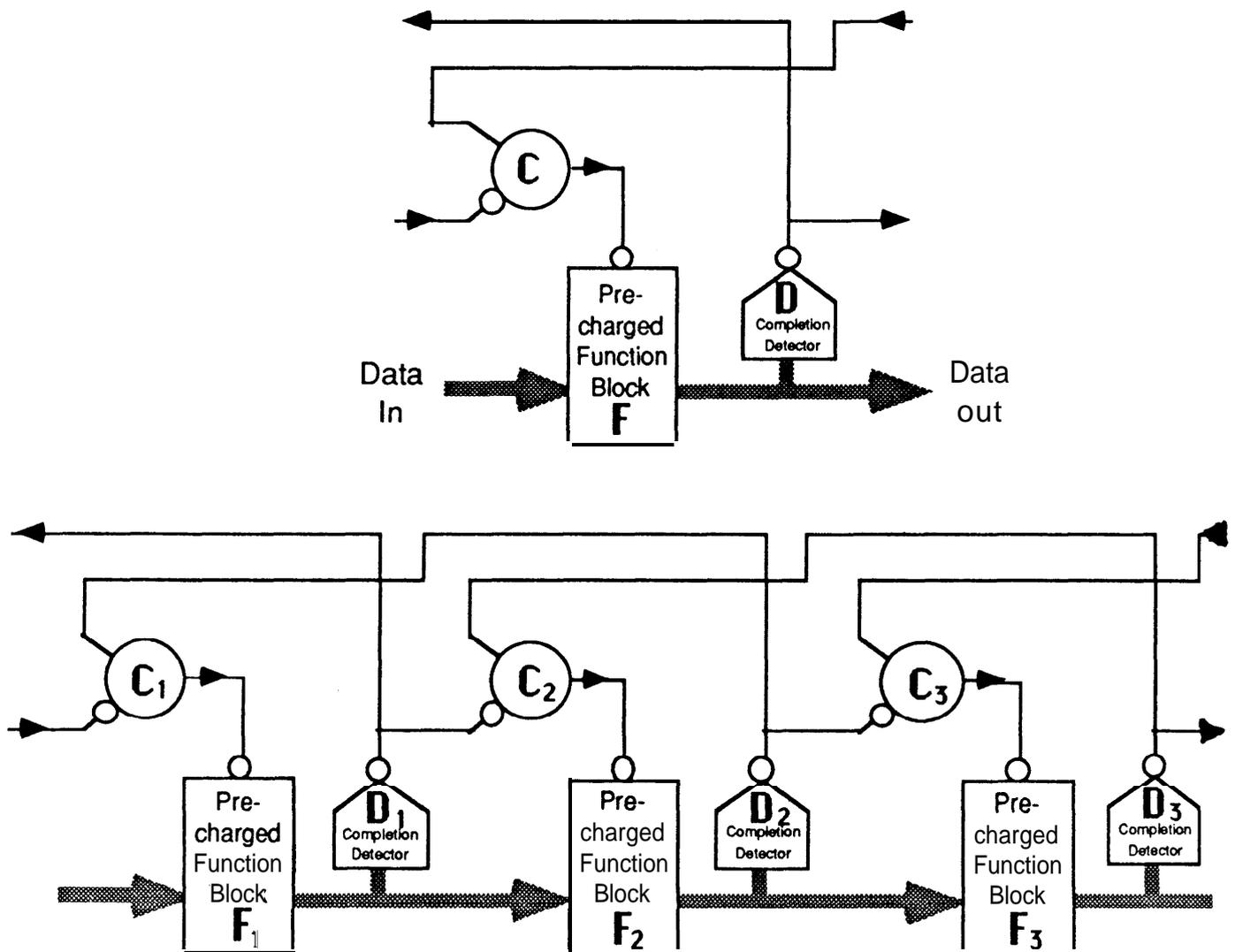
Figure 6: Schematic for stage style **PC0** and a short pipeline composed using that configuration.
