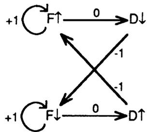
Figure 13: The Folded Dependency Graph for the **PS0** configuration pipeline
