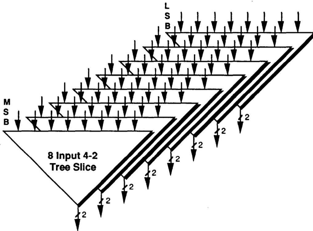
**Figure 3.6 Multiple 4-2 Tree Slices Form a 4-2 Multiplier**
