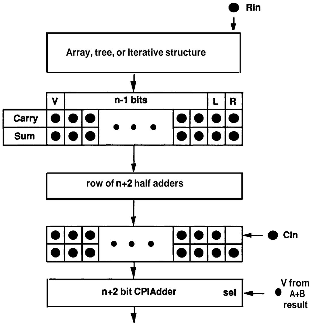
Figure 6.4 Algorithm 6.2A Data Flow
