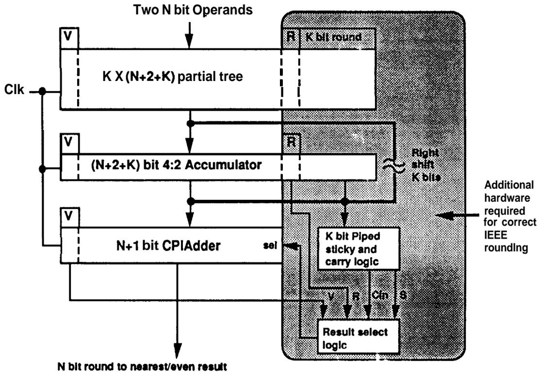
Figure 6.11 SPIM Type Iterative Multiplier with IEEE Rounding
