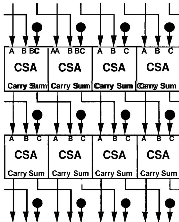
Figure 2.2 Two Rows of an Array Multiplier\*
