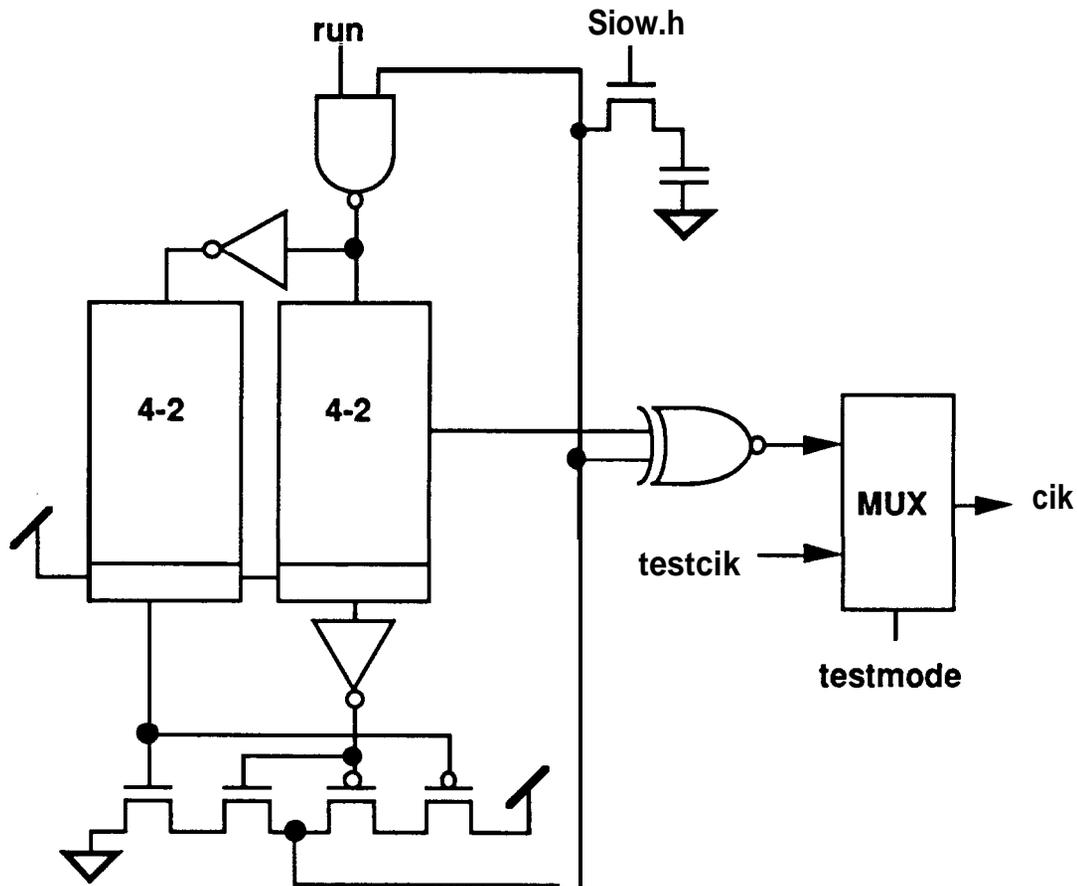
Figure 5.7 implementing A Dual 4-2 Tracking Clock Generator
