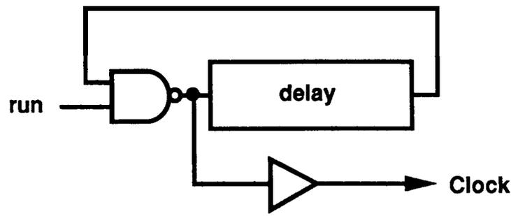
**Figure 5.1 Generic On-Chip Stoppable Clock Generator**
