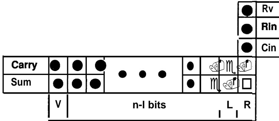
**Figure 6.3 Bits to be Summed for Correct Round to Nearest/up**
