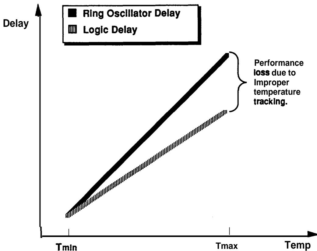
Figure 5.3 Temperature Effects on Tracking
