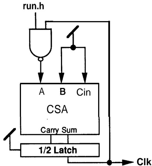
Figure 5.4 A CSA Tracking Clock Generator<sup>14</sup>
