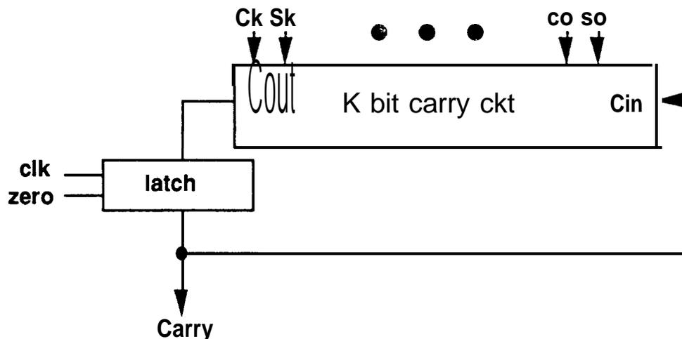
Figure 6.9 Piped Carry Circuit
