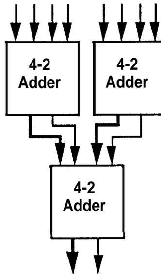
Figure 3.5 An 8 Input 4-2 Tree Slice (Front View)
