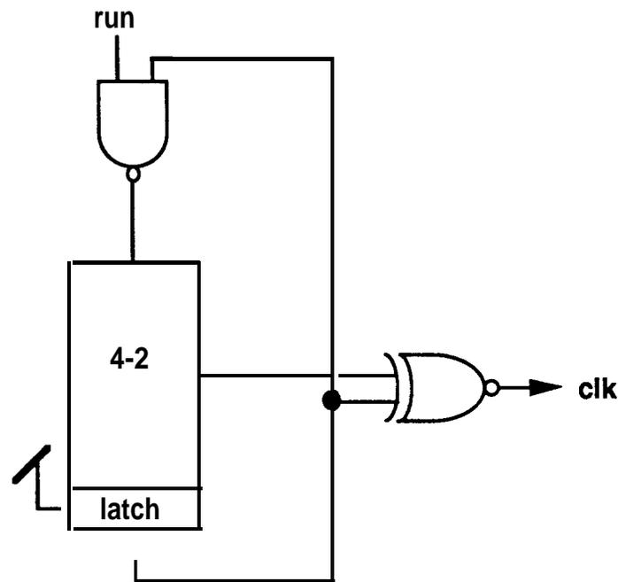
Figure 5.5 A 4-2 Tracking Clock Generator
