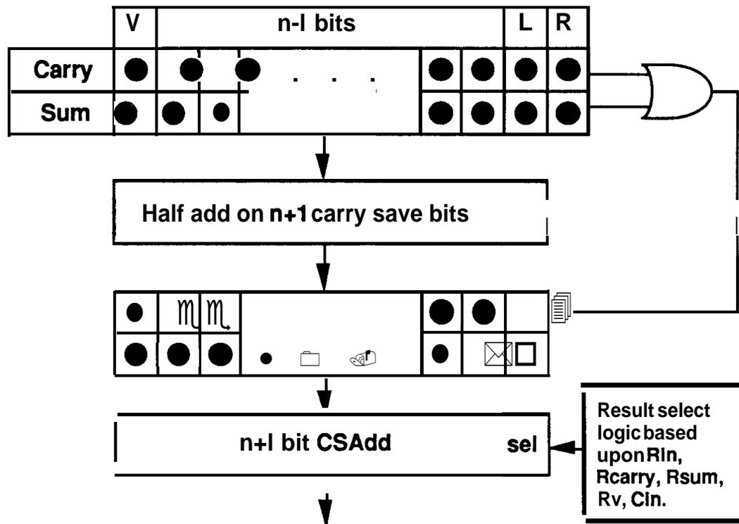
Figure 6.6 Algorithm 6.3 Data Flow
