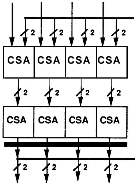
Figure 2.5 Partial Linear Array
