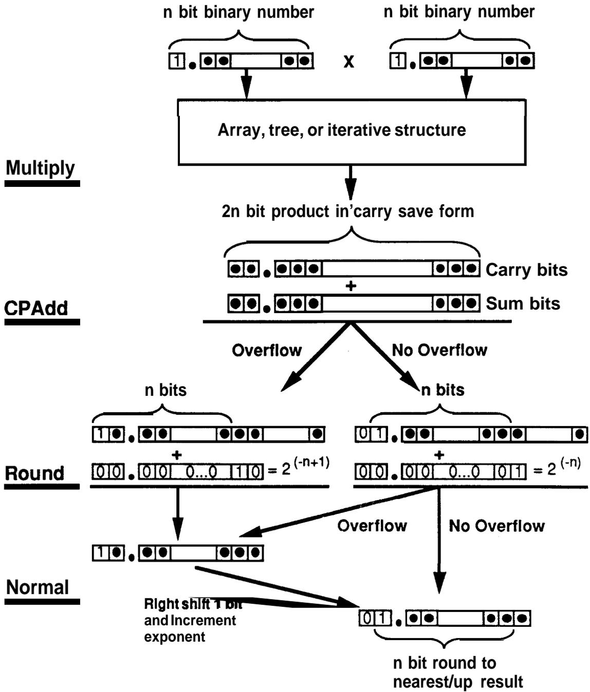
Figure 6.2 Algorithm 6.1 Data Flow
