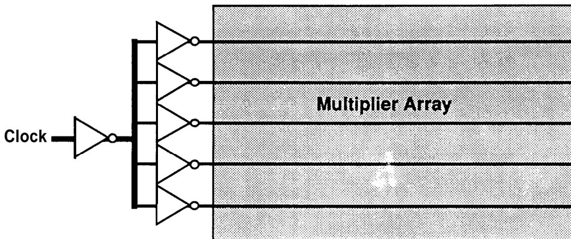
Figure 5.8 Recommended Clock Distribution Across an Array
