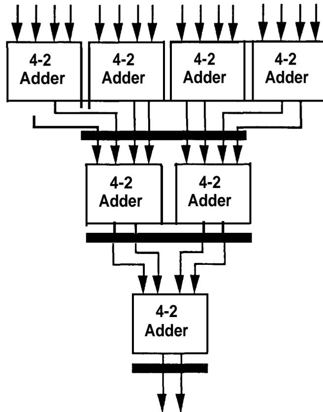
**Figure 3.8** A Pipelined 4-2 Tree
