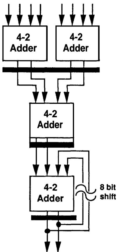
Figure 3.11 An 8 Input Partial 4-2 Tree and 4-2 Accumulator
