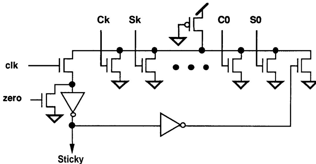
Figure 6.10 Pipelined Sticky Circuit
