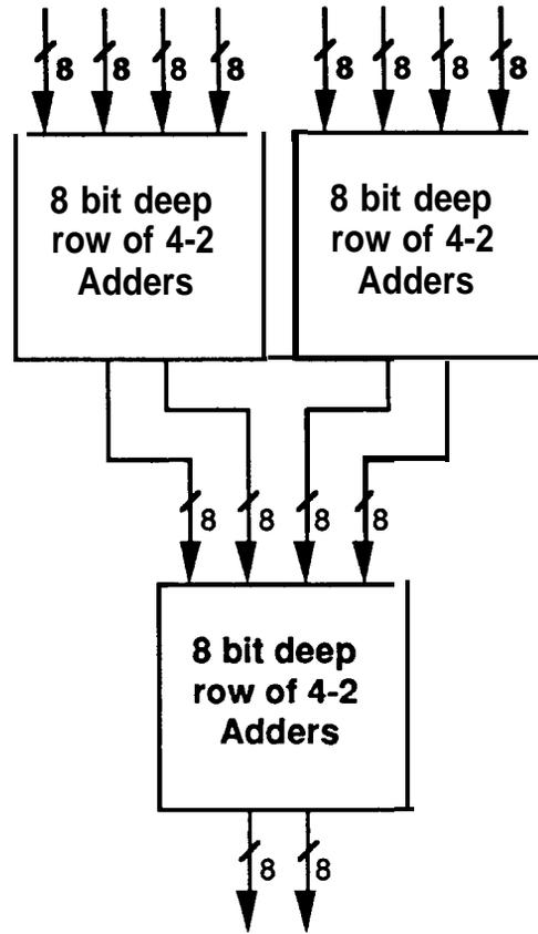
**Figure 3.4 An 8 Input 4-2 Tree (Front View)**
