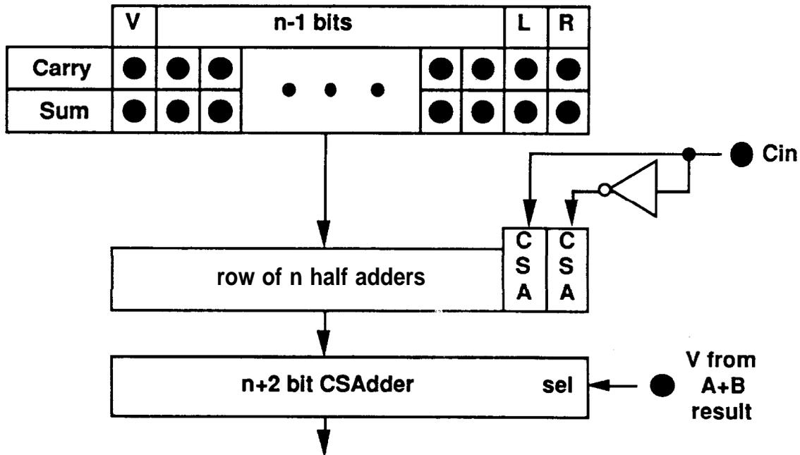
Figure 6.5 Algorithm 6.28 Data Flow
