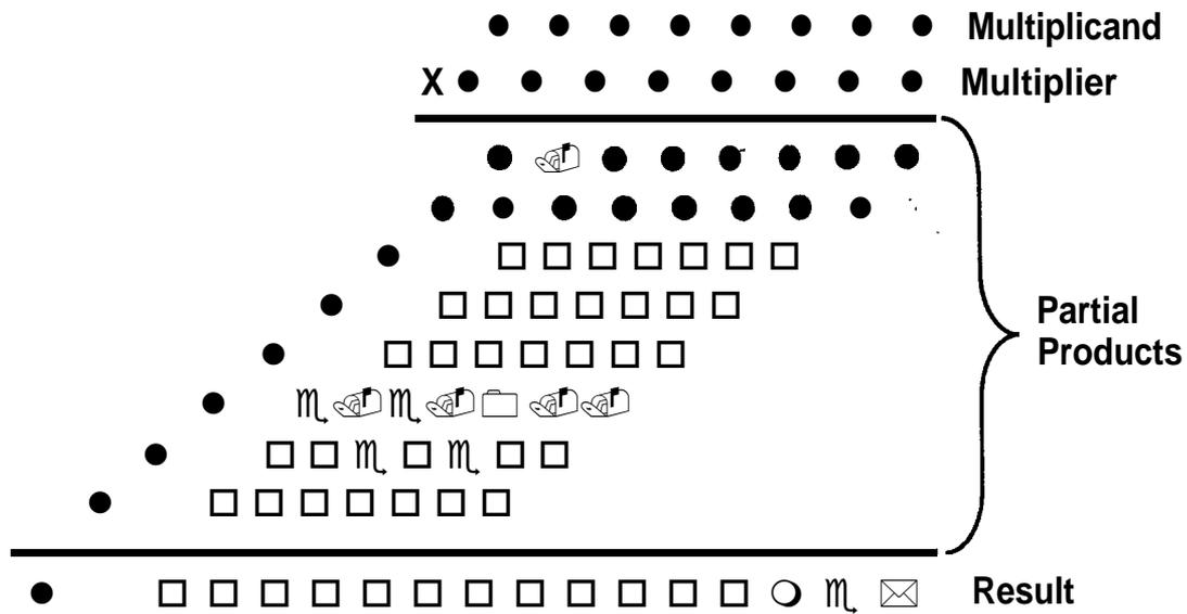
Figure 2.1 Basic Multiplication Data Flow
