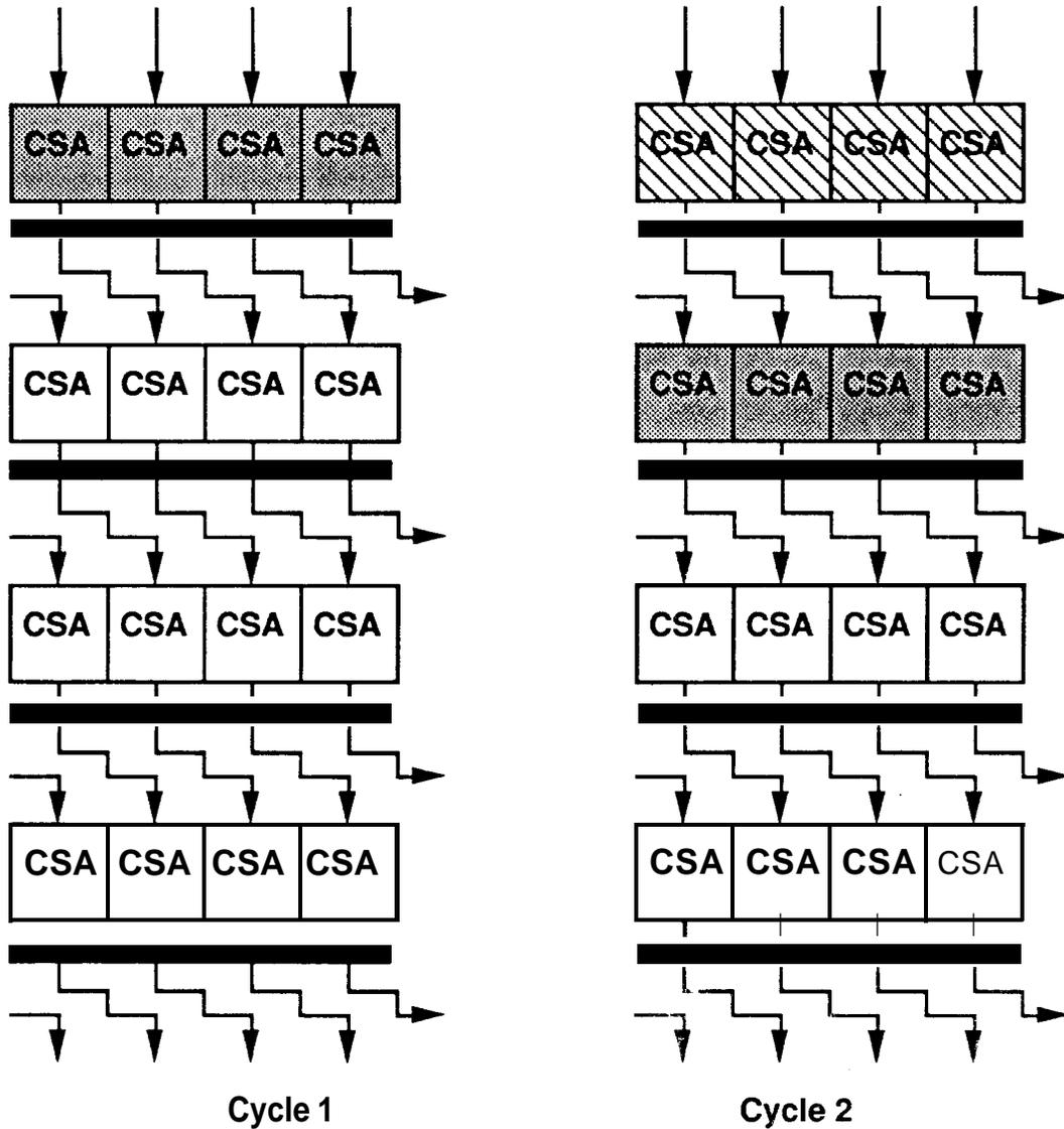
Figure 2.3 Data Flow Through a Pipelined Array Multiplier<sup>4</sup>
