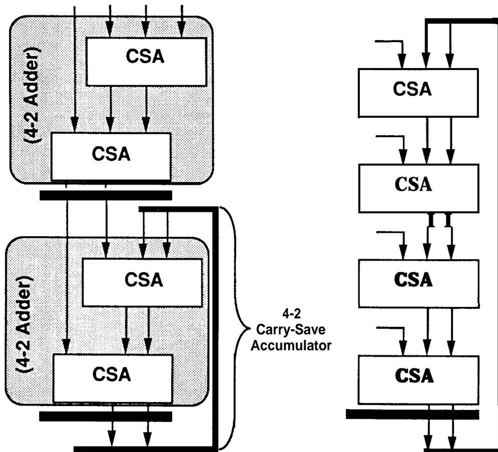
Figure 3.10 4-2 Tree and Accumulator vs. Partial Linear Array
