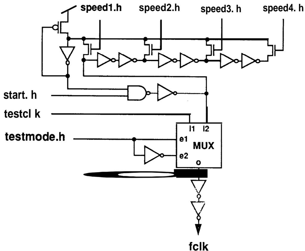
Figure 4.3 The SPIM Clock Generator
