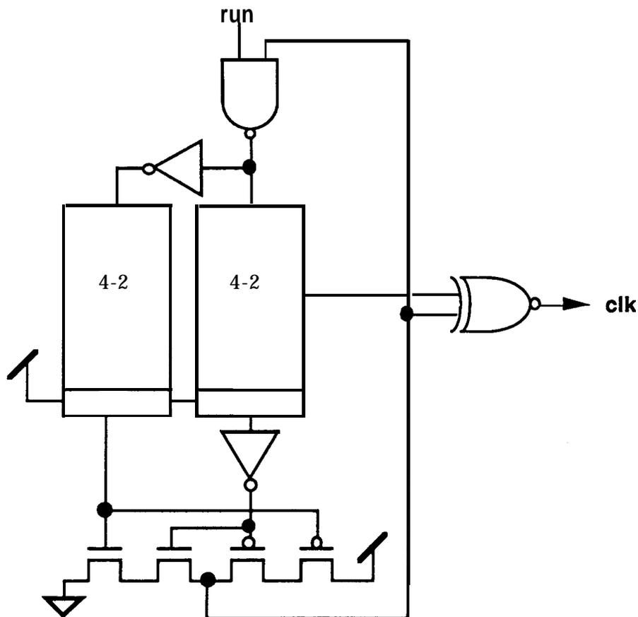
**Figure 5.6 A Dual 4-2 Tracking Clock Generator**
