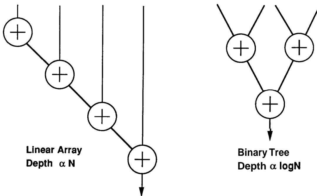
Figure 2.6 Linear Array versus Tree Structure
