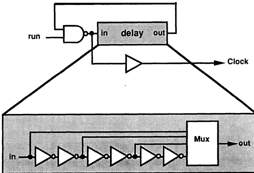
Figure 5.2 Programmable Delay Clock Generator
