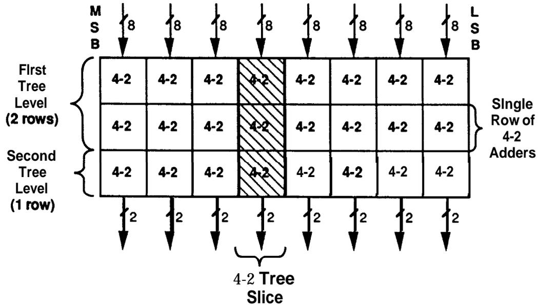
**Figure 3.7 An 8 Bit 4-2 Multiplier Bit Slice Layout**
