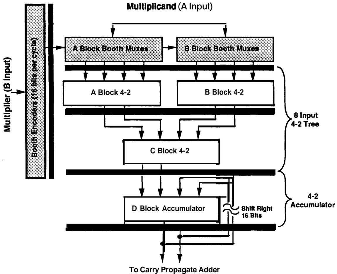
Figure 4.1 SPIM Block Diagram
