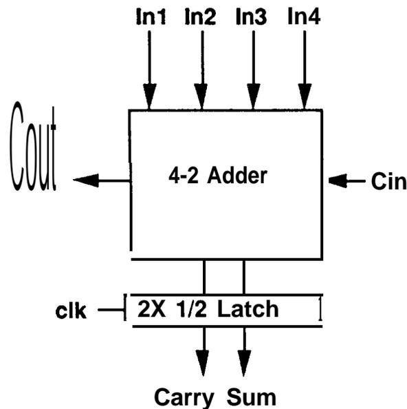
**Figure 5.10 Single Half Latched 4-2 Adder**
