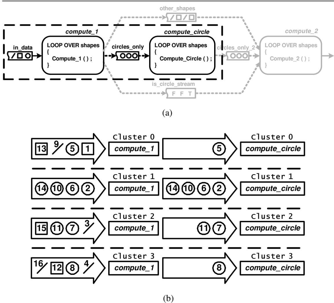
Figure 5.1: Load-imbalance due to conditional routing on a SIMD architecture. The example is based on a portion of the original *shapes* kernel from Section 3.2. Part (a) highlights the portion of the original example which we will focus on in this section. Part (b) shows the execution of the highlighted portion on a SIMD stream machine with four clusters. An example input dataset is given, as well as the results for that dataset.
