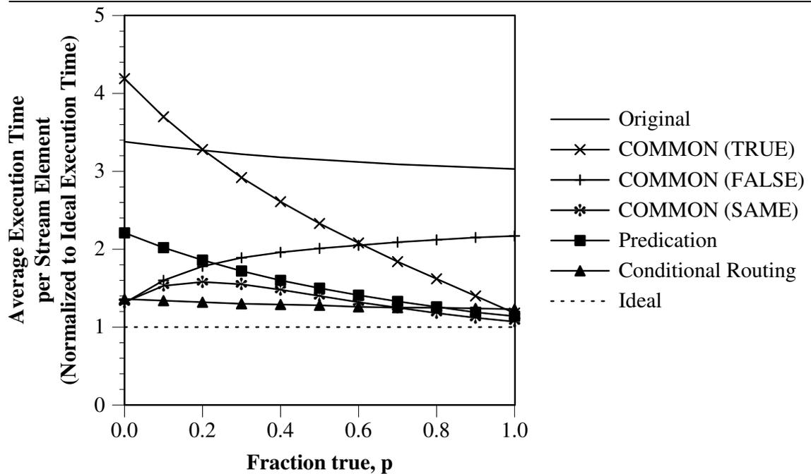
Figure 3.5: Comparison of execution times for existing techniques and conditional routing for the *synthetic\_if* kernel. The execution times are shown normalized to IDEAL.  $W_{\text{body}} = 32$  operations;  $W_{\text{input}} = W_{\text{output}} = 17$  operations;  $S = 2$  words.
