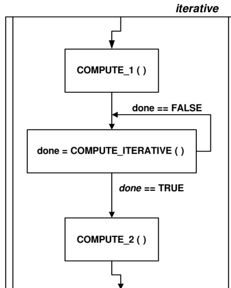
Figure 3.12: An example of a kernel, *iterative*, that contains a while-loop.
