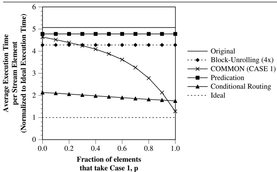
Figure 3.7: This graph shows the results for various conditional techniques on the *synthetic\_case* benchmark. The execution times are normalized to IDEAL. The value of  $p$  in this case indicates how often the first case is taken; the other seven are taken an equal amount of times.  $W_{\text{case}} = 32$  operations,  $W_{\text{input}} = W_{\text{output}} = 17$  operations,  $S = 2$  words.
