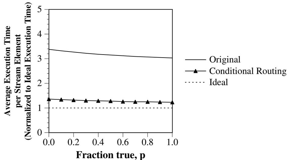
Figure 3.4: Impact of conditional routing on execution time for *synthetic\_if*. The execution times are shown normalized to IDEAL.  $W_{\text{body}} = 32$  operations;  $W_{\text{input}} = W_{\text{output}} = 17$  operations;  $S = 2$  words.
