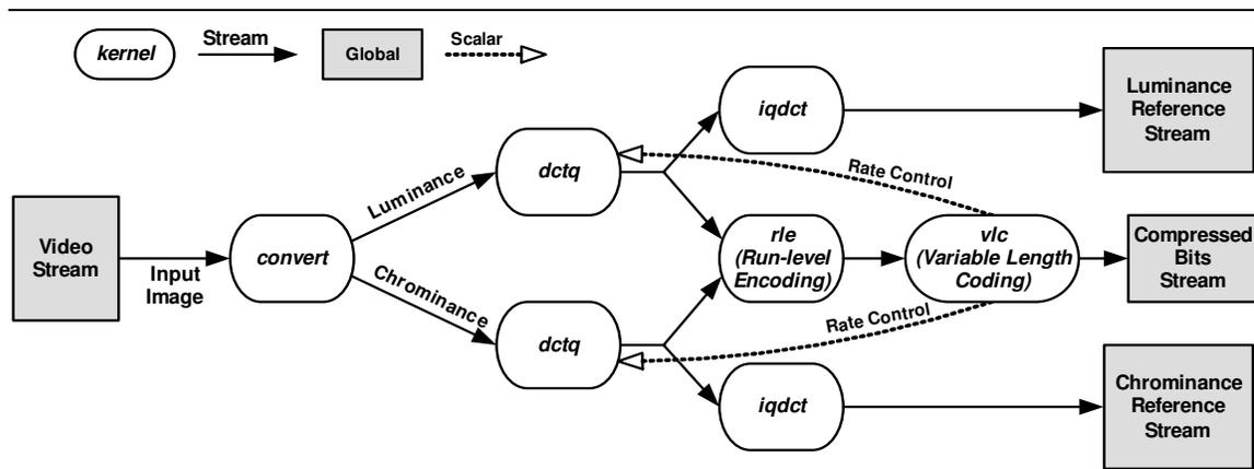
Figure 2.2: MPEG-2 I-frame encoder mapped to streams and kernels. The encoder receives a stream of macroblocks from a frame in the video feed as input, and the first kernel (*convert*) processes these. The discrete cosine transform (DCT) kernels then operate on the output streams produced by *convert*. Q=quantization; IQ=inverse quantization.
