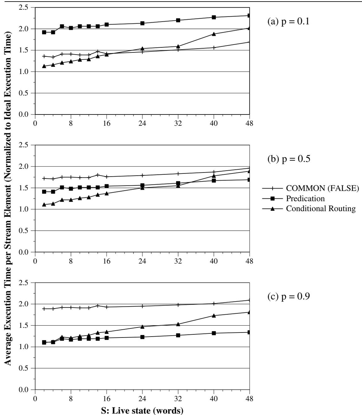
Figure 3.11: These graphs show the impact of increasing the amount of live state,  $S$ , in the *synthetic\_if* kernel on the execution time for the various if-statement techniques.  $W_{\text{body}} = 128$  operations,  $W_{\text{input}} = W_{\text{output}} = 65$  operations.
